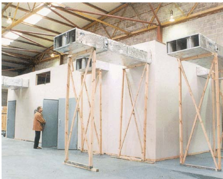
Purpose-built IAC test facility for a 12m 3 /s on-floor AHU.
