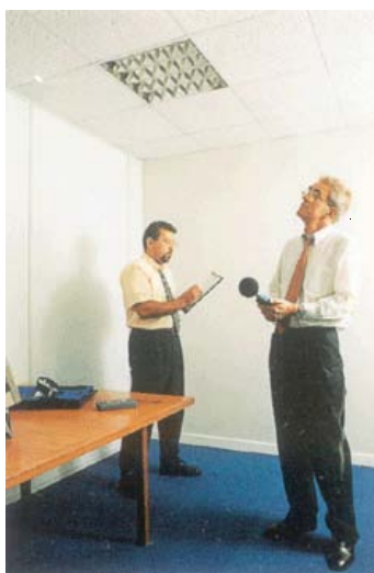
Typical office test in which AHU noise levels are measured.
